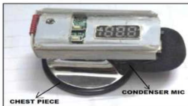
Figure 2b: Wireless Electronic Stethoscope with different parts
